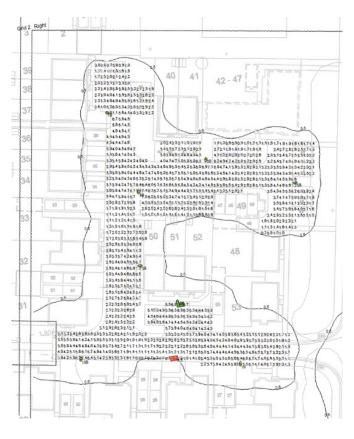
Performance results such as those shown left should be transferred to the base proposal drawings along with evidence of calculation as supporting safety evidence within the clients construction files as required in the Construction, Design and Maintenance Regulations (CDM)
